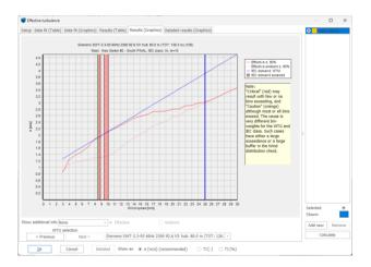
Click OK and the turbulence calculation gets an overall yellow result. Thus, the WTG effective turbulence exceeds the IEC limit for some wind speeds, but not in a critical way.
